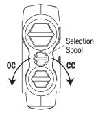
• For closed-center operation, tighten the spool in the clockwise direction until snug.
