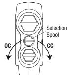
For closed-center operation, tighten the spool in the clockwise direction until snug.
