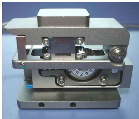
Cleaving Finished Position
