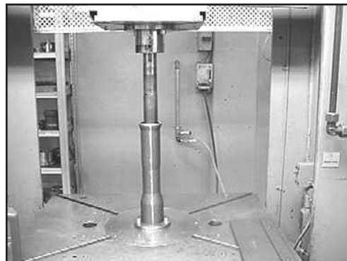
6. Press the bushing into the nose part with a pressure of 10 t.
