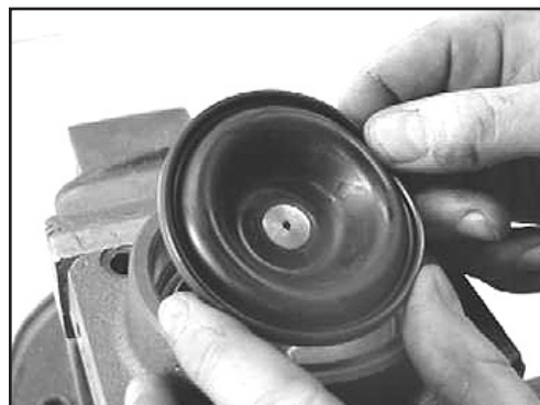
7. Check the diaphragm for defects.
