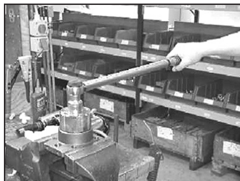
6. Tighten the cover with a hook wrench to 200 Nm (148 ft-lb).
