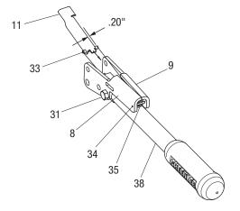
15. Insert shoulder screws (13 and 16) to align handle plates and tighten hex screws (31) to 170-190 in-lb. Remove shoulder screws.
