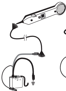
Figure 4a. Cable Tracing
