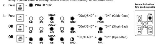
4. Test complete. Go to the next cable test, or perform a "Fault Check" operation to troubleshoot faulty cables. Do not press the "ON/TEST" button. This will turn off the tester and prevent a "Fault Check" from being performed.
