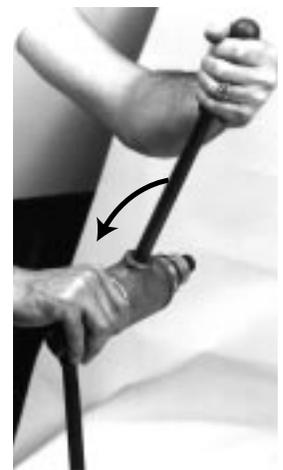
11. For rapid return, hold the assembly as shown. Rotate the handle as shown until the spindle is fully extended.
