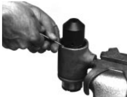
18, 19. Refer to these photos and reassemble in the reverse order. Inspect and reinstall thrust bearings. Install spindle hub unit, wave washer (4), and retaining ring (3). Be sure to seat the retaining ring completely in the groove.
