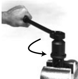
5. Remove hub (7) with ratchet (1) or any suitable 1/2" drive ratchet or breaker bar. The hub was tightened to a torque of 90 ft-lb to 100 ft-lb at the factory. Therefore, a considerable amount of force will be necessary to loosen.
