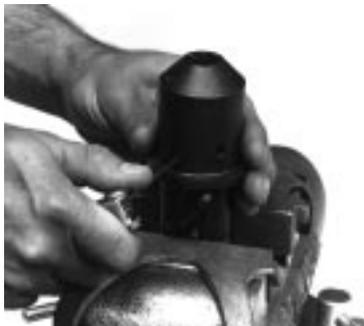
4. Mount unit securely in vise as shown. Care must be taken to not damage ball return tube of the ball nut when gripping with vise. Then remove 3 set screws (6) from unit and discard screws (new screws must be used during reassembly).
