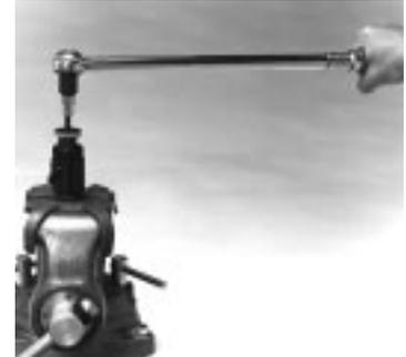
11, 12. Place ball nut with arbor to end of spindle as shown.
