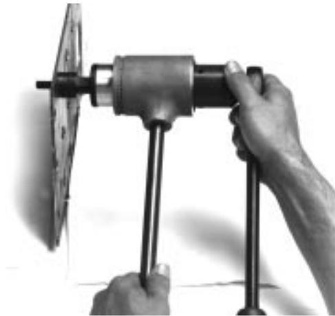
10. Remove the driver assembly from the punched hole.
