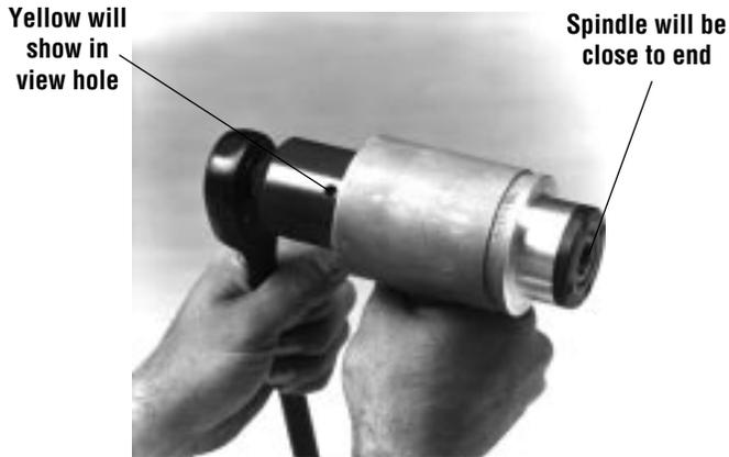
2. Rotate the ratchet as shown. When the spindle is fully extended, the view hole will be completely filled with the yellow band.
