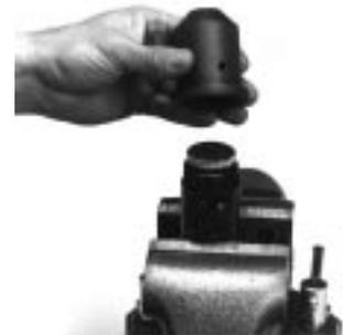
6. Unscrew hub and remove from ball nut.
