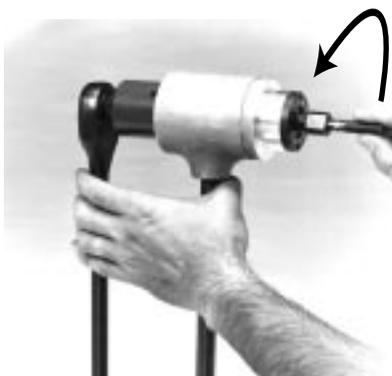
3. Select the appropriate punch and die. Use the Draw Stud Selection Table to determine the corresponding draw stud. Install the draw stud as shown.
