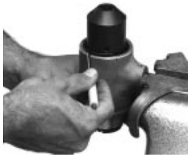
2. To remove retaining ring (3), use small screwdriver to remove tab end of ring from groove and "spiral" ring out of groove as shown in photo.
