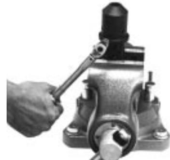
15. Reassemble hub (7) to ball nut. (Note how unit is held in vise.)
