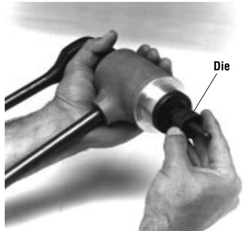
5. Install the die onto the stud so that the opening of the die faces outward.
