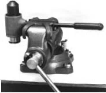
1. Mount unit to be repaired in sturdy vise as shown. Remove ratchet wrench (1) from hub by depressing locking detent with an appropriate tool.
