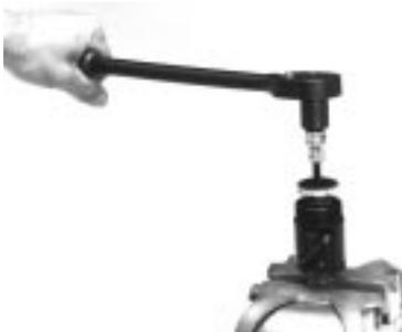
7. To complete disassembly, remove above unit from vise and regrip on "flats" of spindle (13). Use "soft" jaws to prevent damage from hard vise jaws. Loosen flat head screw (8) with Allen wrench and remove top washer (9).
