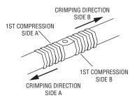
7. Using the sequence illustrated here, pump the handles to advance the dies. Continue to pump until the pressure relief valve activates.
