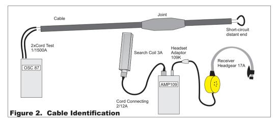
With the Search Coil 3A pointing towards the cable a distinct maximum tone should be identifiable. The strength of the signal will vary as the search coil is moved along the cable; this is because the magnetic field strength varies as the pair of wires cross and as they move around the bundle within the cable.
