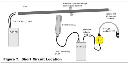
wire of the pair, the currents in the two wires being in opposite directions. To obtain a strong magnetic field the pair should be short-circuited at the far end so that maximum current will flow. As the metal sheath, barrier foil or conductors do not shield the magnetic field to any great extent, the tone may be detected outside the cable. However, steel armouring wires or tapes may reduce the field outside the cable.
