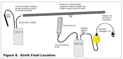
Alternately hold the search coil horizontally (see figure 9), when it points along the route of the cable there should be a null in the received signal and a maximum in the received signal when it points across the direction of the cable. Where an earth fault
