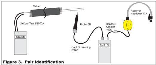
then be found by selecting a section of the joint having the loudest tone. Groups of pairs and finally individual pairs should be eliminated by selection until one pair is found to have the loudest tone. During this process the amplifier gain should be set to give the minimum signal, otherwise the weak tone induced into other pairs may cause confusion.
