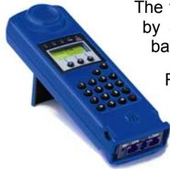
The tester is normally powered by 3 "AA" type rechargeable batteries.
