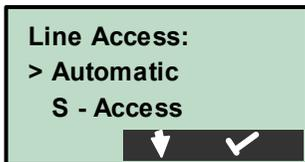
Use the soft-keys to select the required **Line Access** or to scroll down the menu.
